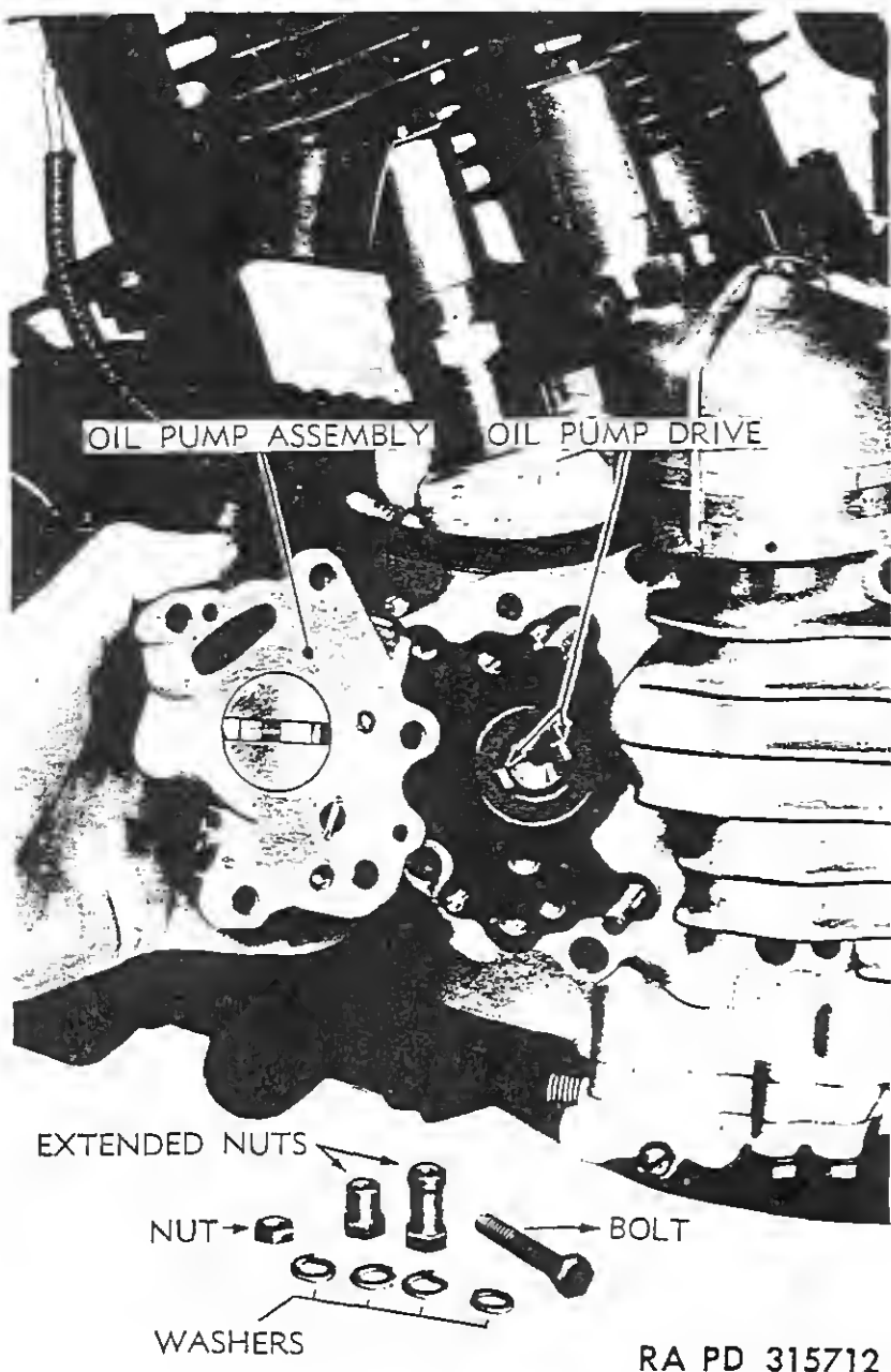
Figure 17—Oil Pump Removed
