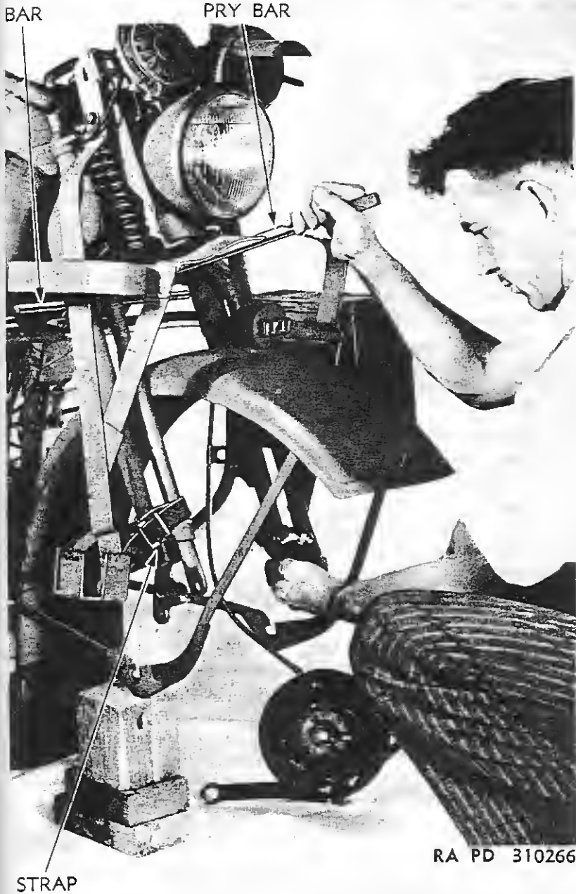
Figure 64—Compressing Cushion Springs for Spring Fork Assembly
